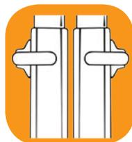
**B. The second mechanical component of the ladder is the LOCK ASSEMBLY.** There are four of these on each ladder.
