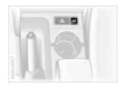
Use this button to operate the central locking system whenever the doors are closed. The doors and luggage compartment lid are unlocked or locked only. The anti-theft alarm system is not activated.
