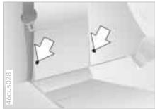
Leave the rear safety belts in the holders if they are not needed to avoid unwanted movement from the safety belts at high speeds.
