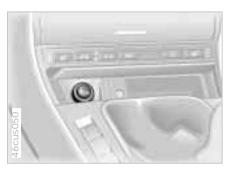
Press the lighter in. As soon as it pops back out, the lighter can be removed.
