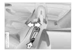
The seat-integrated safety belt allows easy access to the rear. You do not need to adjust the safety belts. They automatically adapt to various body sizes.
