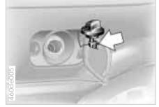
Close the fuel cap carefully after refueling until a "click" is heard. While closing, be sure not to squeeze the strap which is fastened to the cap. A loose or missing cap will activate the Service Engine Soon lamp. ◀
