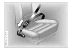
The safety belt tensioner makes sure that the belt tightens during a head-on collision to ensure that occupants remain firmly positioned in their seats. A gas-pressure system retracts the buckle assembly to tension the shoulder and lap belts within fractions of a second. This reduces the tendency to slide under the lap belt.
