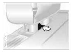
If, after being automatically triggered, the protective function is not needed, then the rollover protection system can be lowered back into place. No special tool is needed for this.
