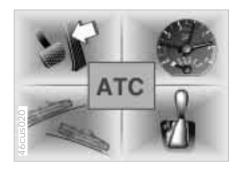
On vehicles with automatic transmission, the Adaptive Transmission Control (ATC) uses a number of factors to calculate the most efficient gear. In this process, it considers your individual driving style as well as current driving conditions.
