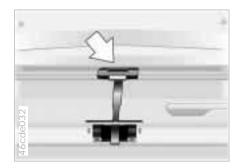
3 Raise and secure the floor panel by hanging it from the rubber seal ring for the run-off gutter (arrow).
