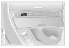
3 From ignition key position 1 on press the switch to unlock the convertible top. The convertible top unlocks and opens slightly. The side windows lower slightly.
