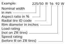
The speed rating indicates the approved maximum speed for the tire.
