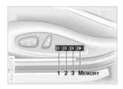
You can store and recall three different driver's seat and exterior mirror positions. The illustration shows the buttons on the driver's seat for making these adjustments.
