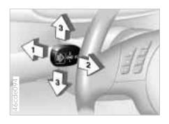
Press the lever up to but not beyond the detent. It will then return to the center position when released.
