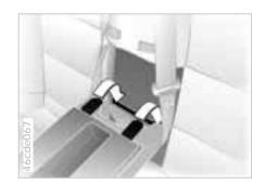
When reattaching the filler piece, guide both bars into the guide and press the filler piece back into place. Secure the safety belts in their holders again. ◀
