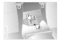
If the mechanisms for the convertible top compartment lid do not unlock, then insert the Allen wrench (1) into the recess (2) and turn clockwise until the mechanisms unlock. ◀
