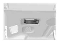
The OBD interface socket for onboard diagnostics is located on the driver's side, on the left-hand bottom of the instrument panel and under a cover panel. The cover is marked with the letters "OBD".
