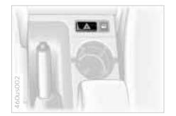
The button flashes on and off when the hazard warning flashers are on.
