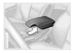
To open the storage compartment in the front center armrest: press the button (arrow) and lift upward.
