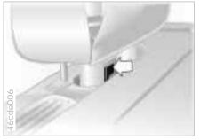
2Pull the lever (arrow) toward the front of the car and hold it in this position.
