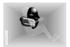
Deceleration sensors continuously monitor the acceleration forces acting upon the vehicle. If, as the result of a frontal collision, a deceleration is reached at which the protection of the safety belts alone is no longer adequate, the gas generators of the driver and passenger-front airbags are ignited. However, the passenger-side airbag is only triggered if an additional sensor has recognized that the passenger seat is occupied.
