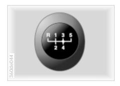
Press the clutch pedal all the way down each time you shift, pressing the manual-shift gear lever into its proper end position.
