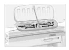
The onboard tool kit is located in the luggage compartment lid.
