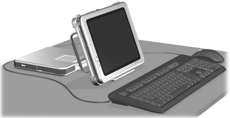
*Tablet PC correctly docked with the keyboard attached*
