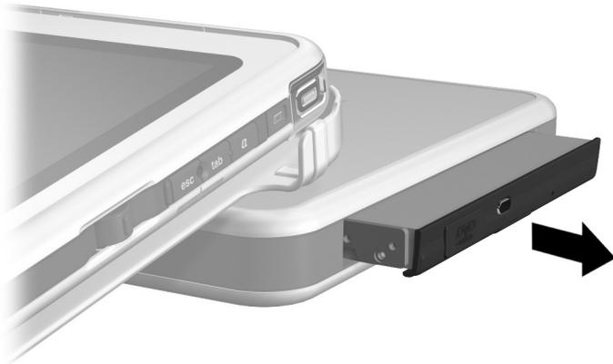
*Removing a MultiBay device*
