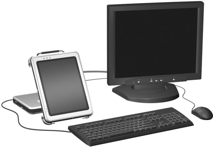
*Tablet PC docked in viewing mode with external monitor, keyboard, and mouse*
