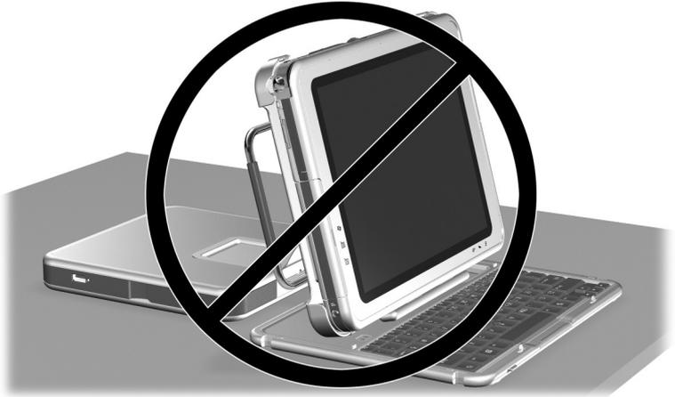
*Tablet PC incorrectly docked with the keyboard attached*
