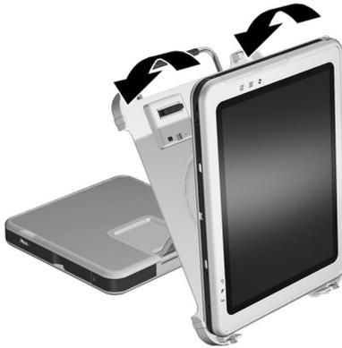
*Aligning and positioning the docking connectors in the portrait position*
