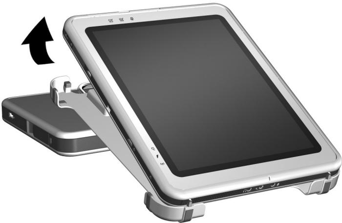
*Removing the tablet PC from the docking stand*
